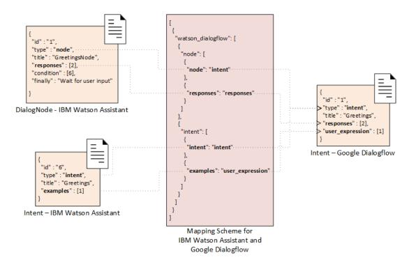
Figure 5.13: Example of a possible mapping scheme for *IBM Watson Assistant* and *Google Dialogflow*
