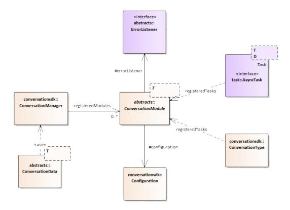
Figure 5.6: System architecture of Conversation SDK
